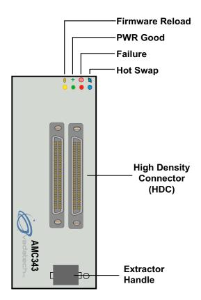
FIGURE 2. AMC343 Front Panel
