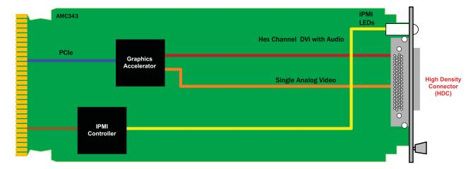
Note: A breakout adapter cable is needed to take advantage of the hex displays. See ordering options for details.
